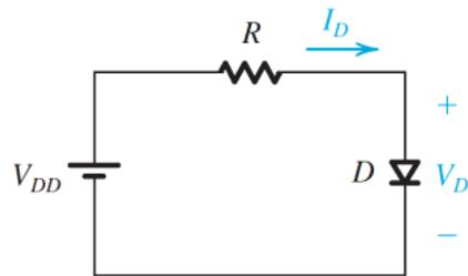
FIG 1. A simple diode circuit
