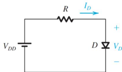
FIG 1. A simple diode circuit
