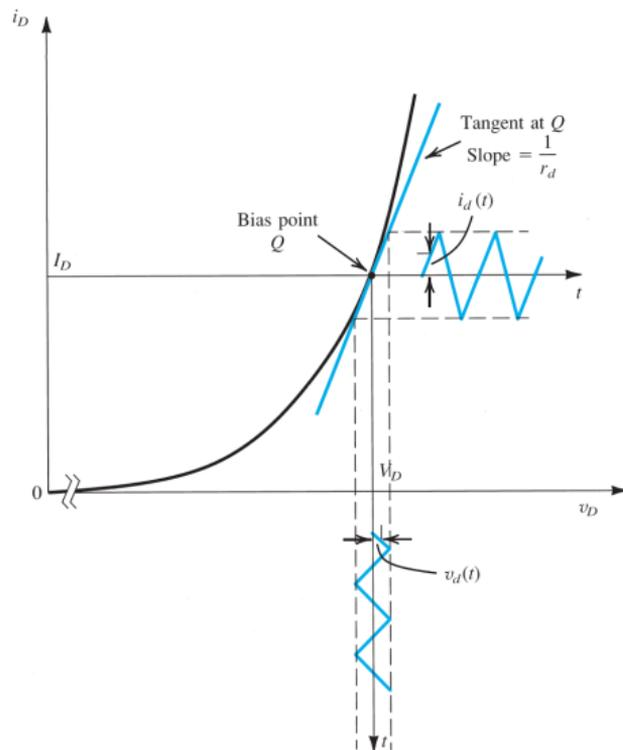
**FIG 7.** The diode small-signal model
