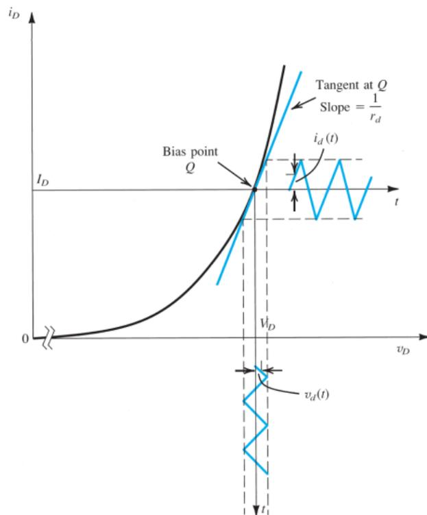
**FIG 3.** The diode small-signal model.
