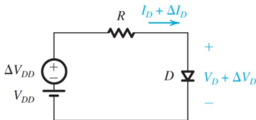
FIG 2. When  $V_{DD}$  changes by  $\Delta V_D$
